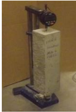
Figure 23 Length measurements of concrete specimens
